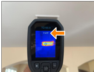
A. Item 4 HVAC temperature and heat mode, 114°
